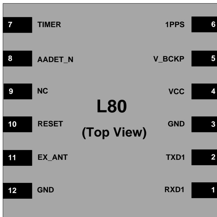
Figure 2: Pin Assignment
