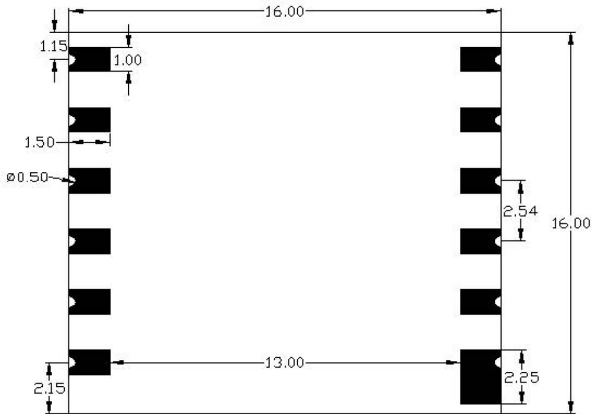
Figure 27: Bottom View Dimensions (Unit: mm)
