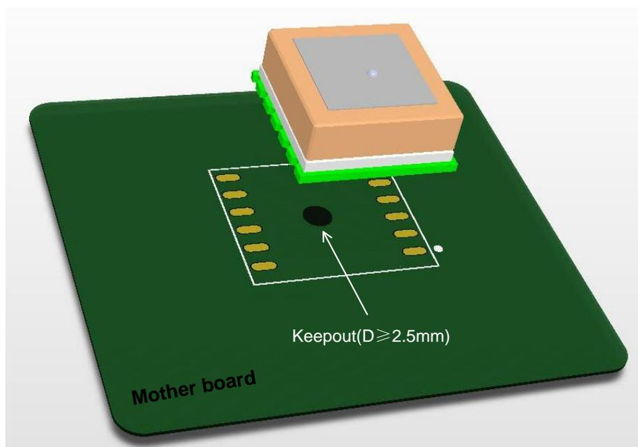
**Figure 19: Recommended Treatment for the Feed Point of the Patch Antenna**
