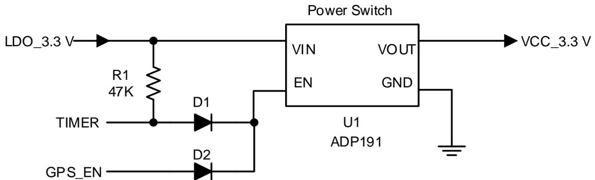
**Figure 6: The External Switch Circuit for TIMER**
