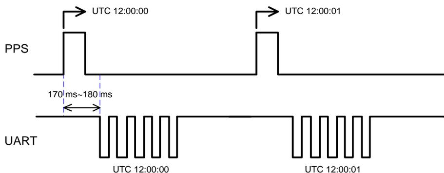
**Figure 16: PPS VS. NMEA Timing**
