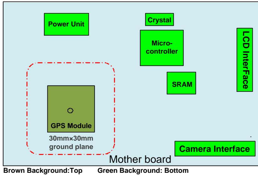
**Figure 22: Recommended Placement of GNSS Module**
