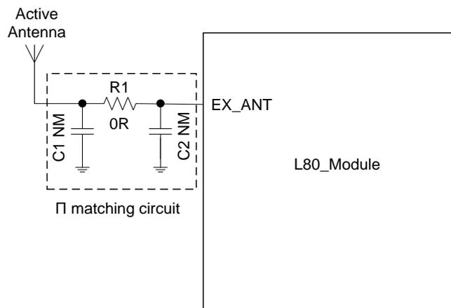
**Figure 24: Reference Design for Active Antenna**
