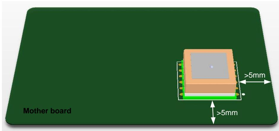
**Figure 18: Recommended Distance between Module and Motherboard Edges**
