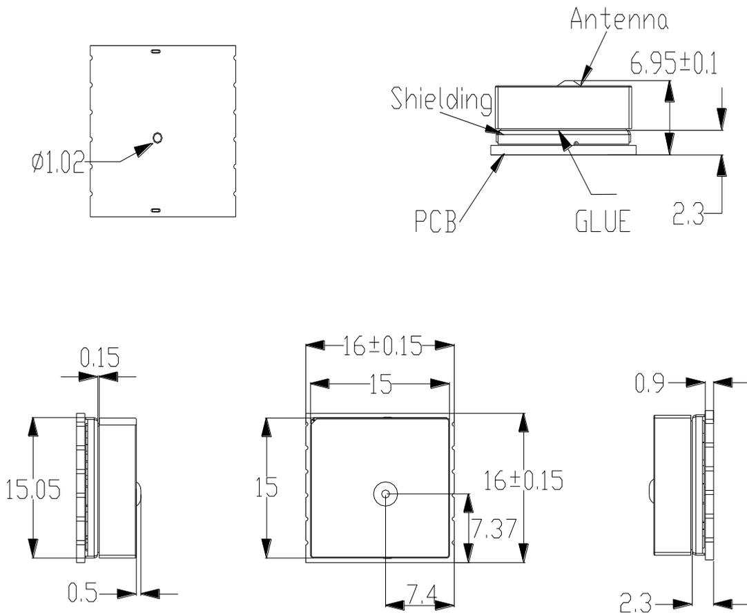
**Figure 26: Mechanical Dimensions (Unit: mm)**
