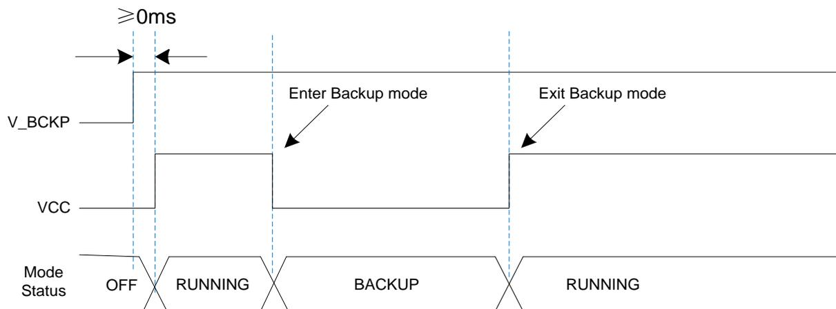
**Figure 7: Backup Mode Sequence Diagram**
