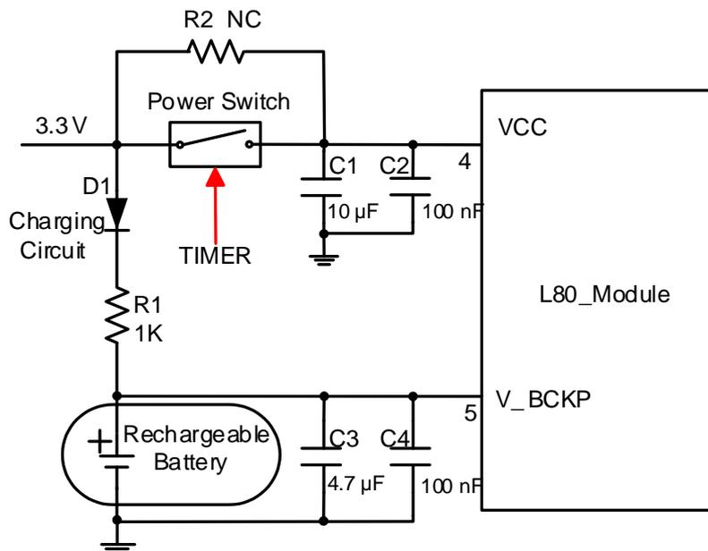
**Figure 5: Reference Charging Circuit for Rechargeable Battery**
