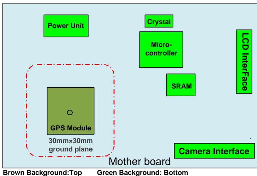
**Figure 23: Recommended Placement of GNSS Module with the RF System**
