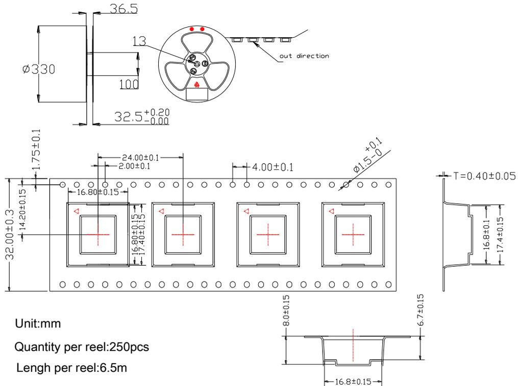
**Figure 32: Tape and Reel Specifications (Unit: mm)**
