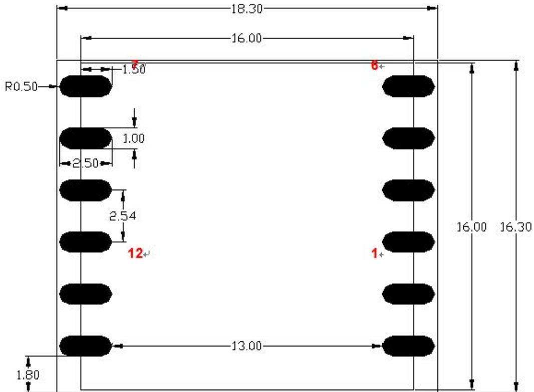
Figure 28: Recommended Footprint (Unit: mm)
