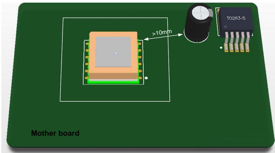
**Figure 21: Recommended Distance between Module and Tall Metal Components**
