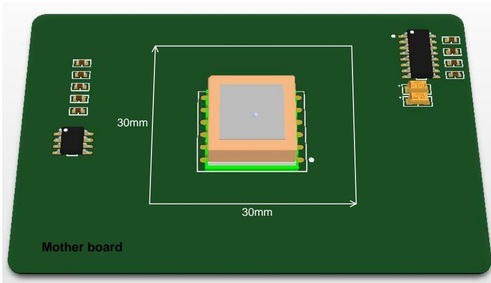
**Figure 20: Recommended Ground Plane**
