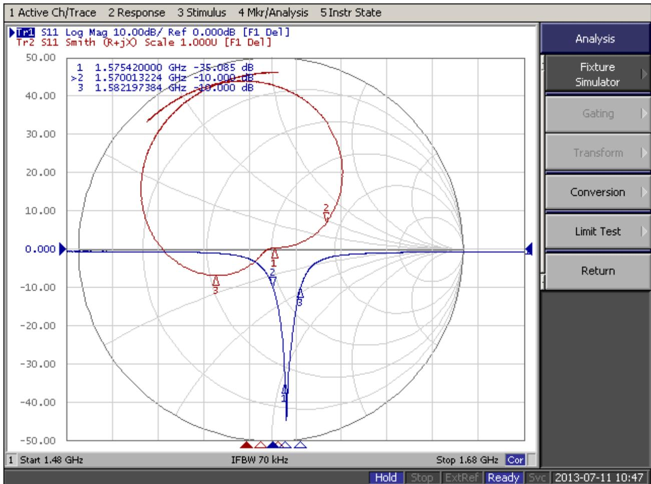
Figure 17: Patch Antenna Test Result with Ground Plane 100 mm × 60 mm
