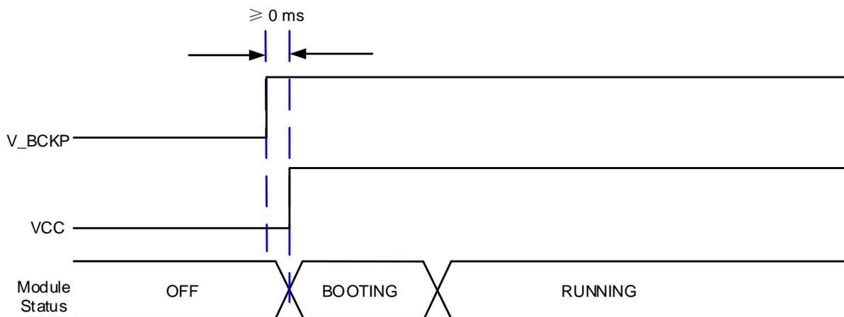
**Figure 11: Power-on Timing**
