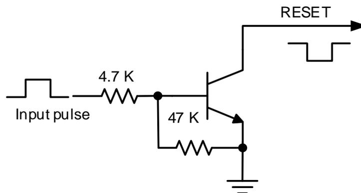
**Figure 12: Reference Reset Circuit Using OC Circuit**
