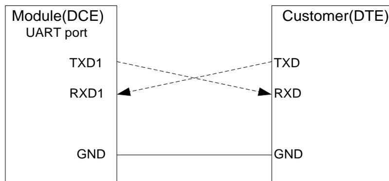
**Figure 14: Connection of Serial Interfaces**
