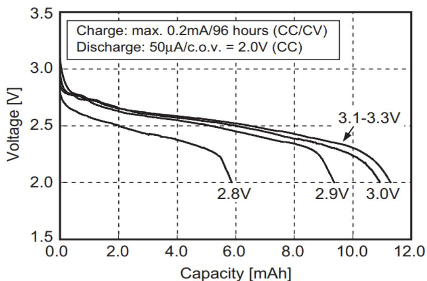
**Figure 8: Seiko MS920SE Charge and Discharge Characteristics**
