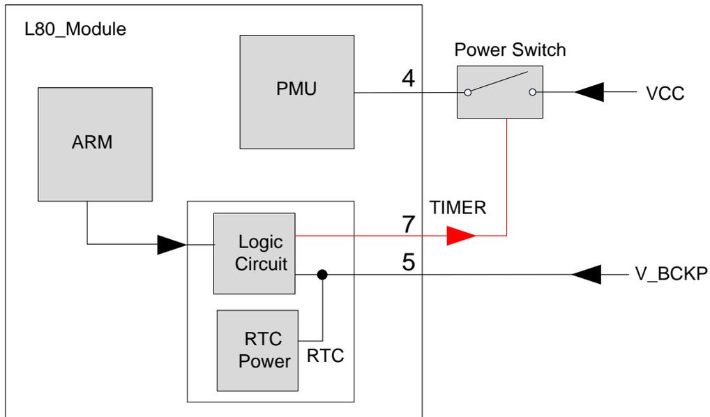
**Figure 3: Internal Power Construction**
