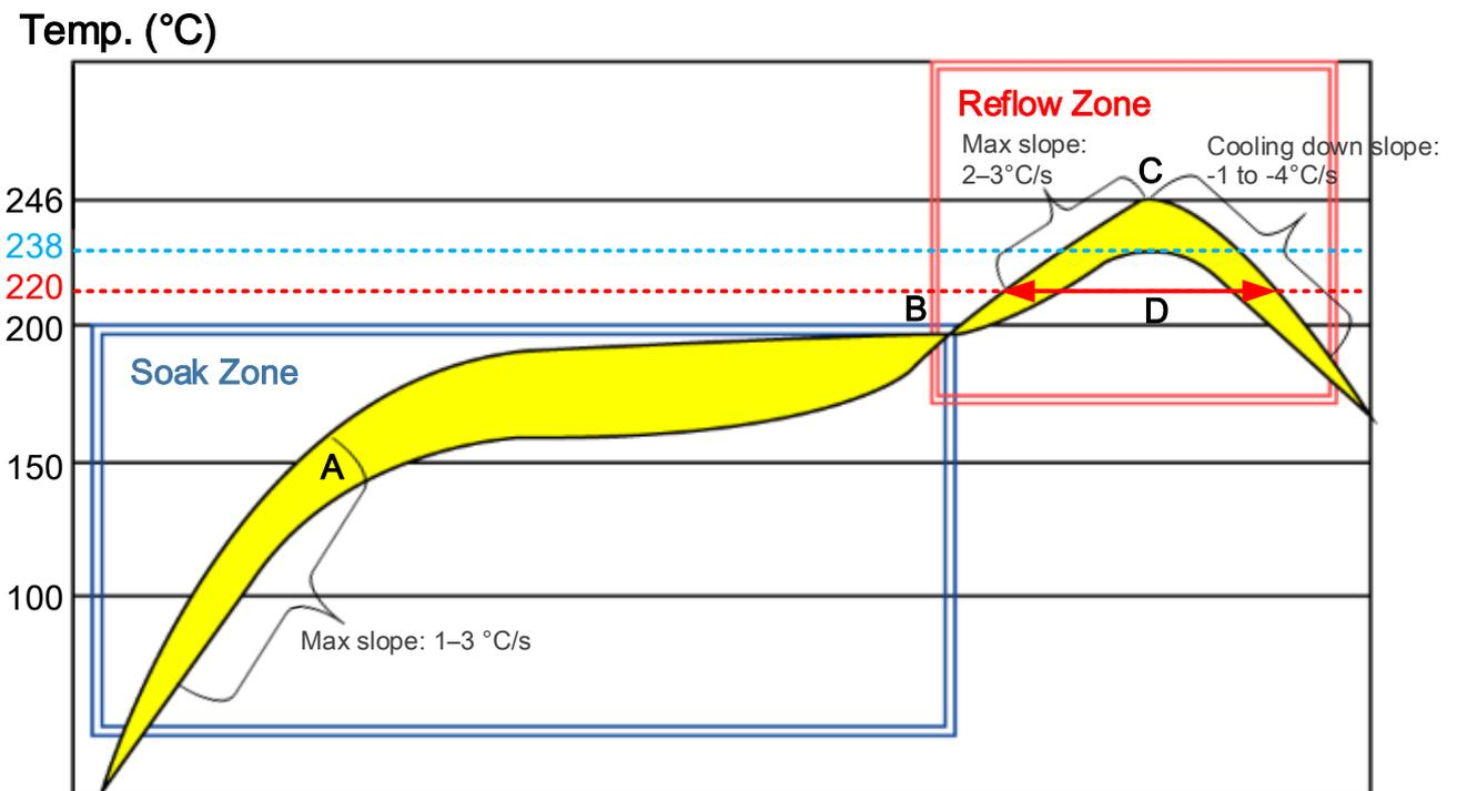
Figure 31: Recommended Reflow Soldering Thermal Profile
