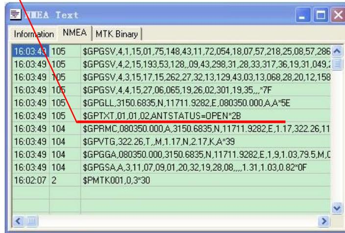
**Figure 25: Patch Antenna Status Description in GPSTXT**
