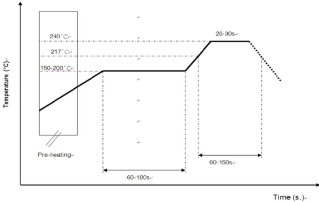
\*Recommended solder paste alloy: SAC305 (Sn96.5 /Ag3 /Cu0.5) Lead Free solder paste.
