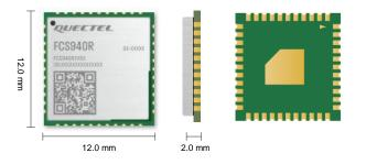
FCS940R is a high-performance 2.4 GHz Wi-Fi 4 and Bluetooth module in LCC package with an ultra-compact form factor of 12.0 mm × 12.0 mm × 2.0 mm. It enables seamless WLAN and Bluetooth connectivity and is designed to optimize end-product size and cost. It incorporates reliable SDIO 2.0 and HS-UART interfaces to provide robust WLAN capability.
