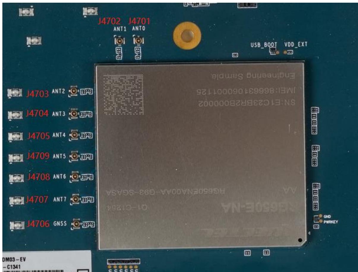
Figure 16: Sub-6 and GNSS Antenna Interfaces
