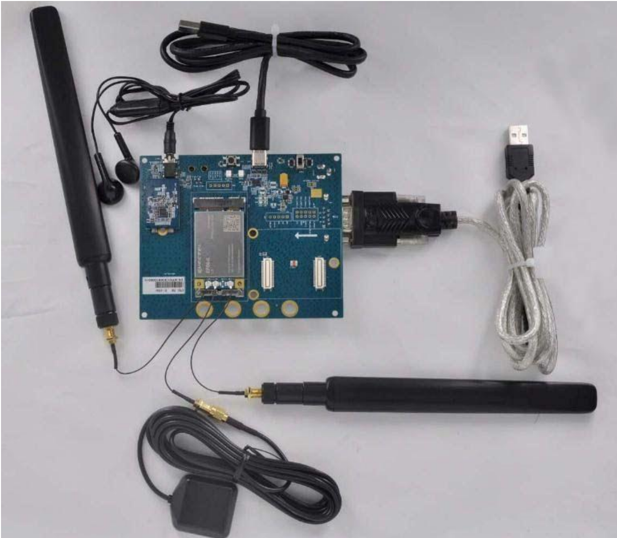
Figure 5: EPXX EVB Kit Accessories Assembly
