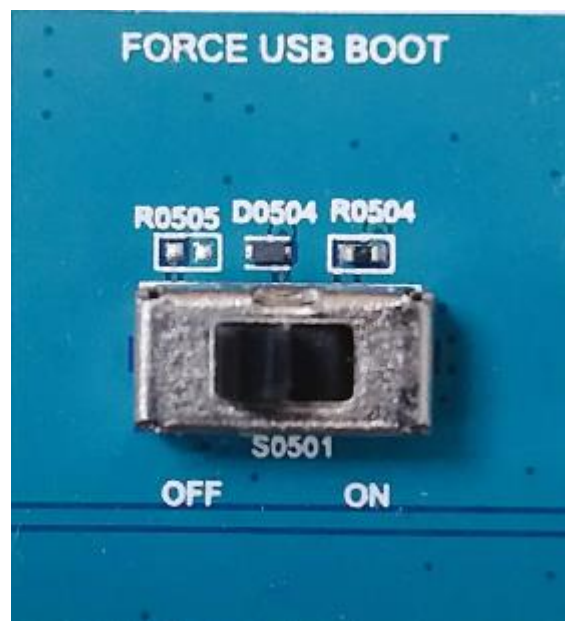
Figure 43: Emergency Download Switch
